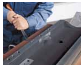
Scraping of Slideway
